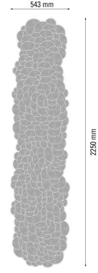
Material: Stainless Steel Thickness: 0,3mm Weight: <2,1 Kg Surface Finish: Gloss Packaging: Cardboard cylinder
